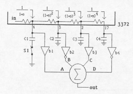
The complex representation of the transfer function of a 1-pole low pass filter is:=  $\frac{1}{1+s}$  Therefore, the transfer function of the network will be:
