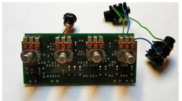
Note that the pots mount on the back (solder-side) of the PCB!
