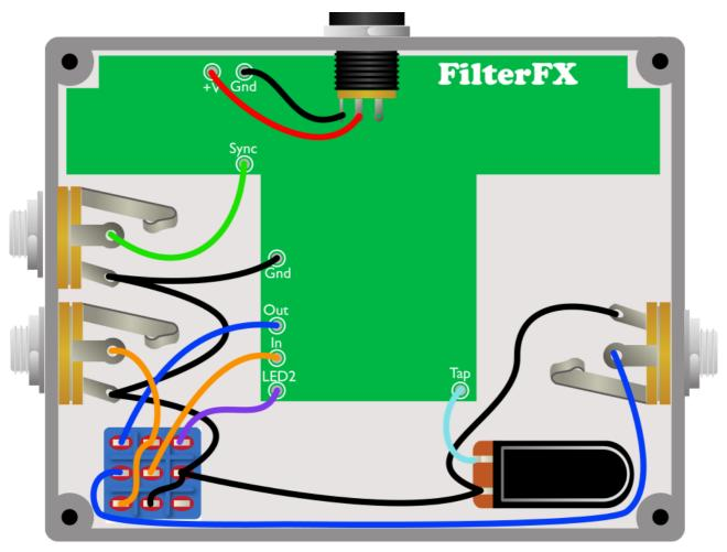
There's a power input and mono I/4" jacks for the input, the output, and the sync input. The two switches are a 3PDT stomp switch to provide true bypass switching and control the bypass LED to show you the on/off status of the effect and a SPST momentary foot switch for the tap tempo.
