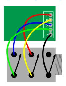
The optional Expression/CV input allows you to connect an expression pedal or CV source to replace the Frequency control of the filter. A stereo/TRS jack with normally closed contacts should be used. The wiring required is shown on the left. Note the T,R,S pads connect to Tip, Ring, and Sleeve connections on the jack. +5 and CV provide the normally connections for Ring and Tip respectively.
