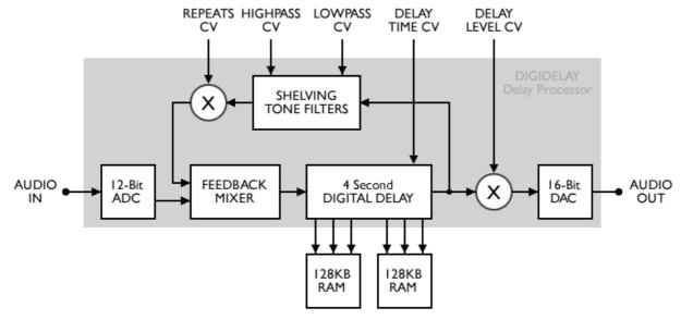
The REPEATS CV, HIGHPASS CV and LOWPASS CV affect the number of repeats and their tone. The DELAY LEVEL CV affects the overall output level of the chip. Note that there is no digital path for the dry signal - the dry signal must be analog, and needs to be mixed outside the chip.
