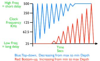
The Depth control introduces LFO modulation into the clock. The modulation is unipolar and can either be introduced from the "bottom up" - e.g. from the longest delay time towards the shortest, or "top down", from the shortest delay towards the longest.
