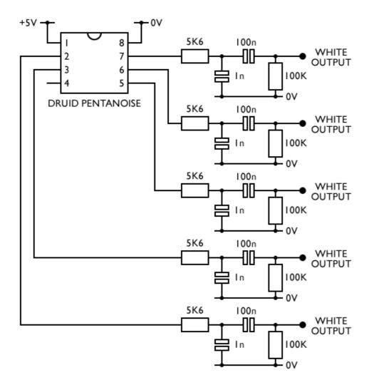
The I48KHz digital noise outputs from the chip are followed by a RC lowpass filter (5K6/In gives Fc=28KHz) and a RC highpass filter for DC blocking (100n/100K gives Fc=15Hz). Because of the highpass filter, each output will take 50msecs to settle at turn on. Outputs levels are approximately  $\pm$ -2.5V (e.g. 5Vpp around 0V).
