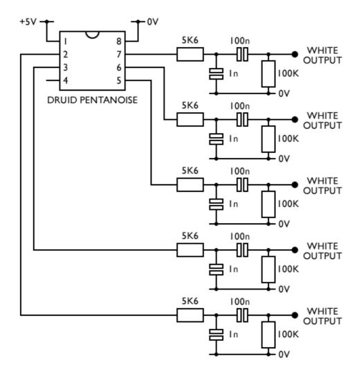
The I48KHz digital noise outputs from the chip are followed by a RC lowpass filter (5K6/In gives Fc=28KHz) and a RC highpass filter for DC blocking (I00n/I00K gives Fc=I5Hz). Because of the highpass filter, each output will take 50msecs to settle at turn on. Outputs levels are approximately +/-2.5V (e.g. 5Vpp around 0V).
