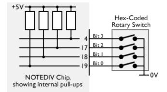
An alternative to hard-wiring the NOTE SELECT pins would be to use a hex-coded rotary switch to select the input. This is easy to do and might be useful in some situations.
