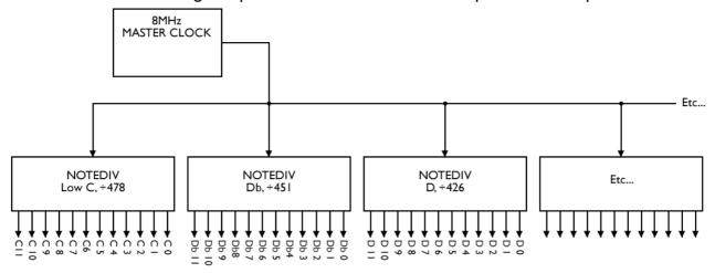
Note the higher clock frequency too - this provides the higher output frequencies which the original chips couldn't manage.
