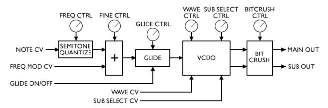
The chip contains 20 waveforms, most of which you're unlikely to have seen before. There are six controls (abbreviated to CTRL above), plus four CVs and one digital input to switch glide on and off. Final output frequency is based on the NOTE CV, the FREQ MOD CV and the FREQ CTRL and FINE CTRL, which gives plenty of scope for control.
