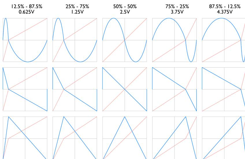
The top row shows the effect of the WAVE DISTORT CV on the SINE wave, whilst the following rows show the effect on the RAMP DOWN and TRIANGLE waveforms. Other waves (excepting RANDOM) are affected similarly.
