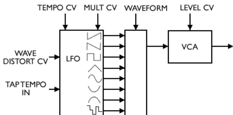
The WAVEFORM voltage selects one of the 8 waveforms. The LFO waveforms can be modified by the WAVE DISTORT CV. Finally, the LEVEL CV sets the output level.
